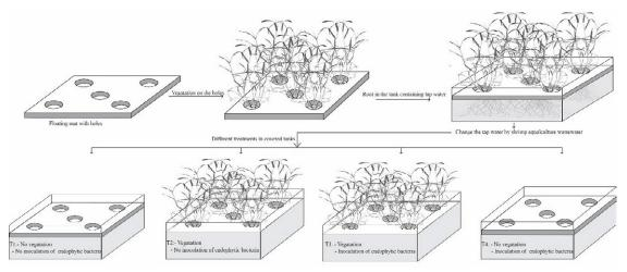
Fig. 1 Different components of floating treatments wetlands and experimental setup
