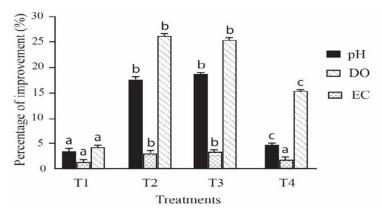
Fig. 2 Percentage improvement of pH, EC, and DO of shrimp aquaculture wastewater after two weeks with different treatments. (T1) sewage wastewater without vegetation and bacterial inoculation, (T2) sewage wastewater with vegetation only, (T3) sewage wastewater with bacterial inoculation only. Each value is mean of three replicates. Different letters indicate statistically significant differences between treatments at a 5% level of significance.
