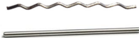
Figure 2. RCSed stainless 316l sample drawing
