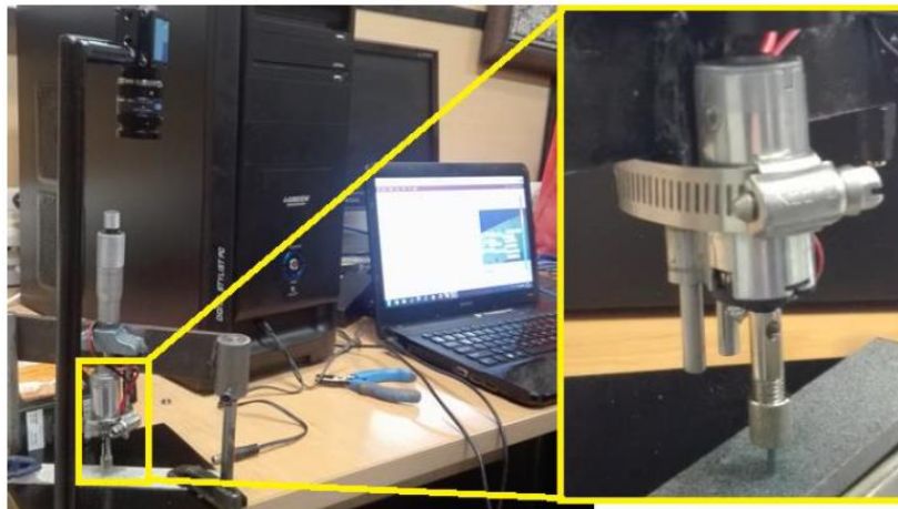
Figure 7. Designed setup for residual stress measurement
