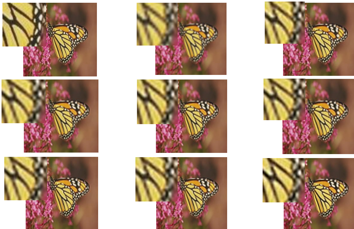
Fig. 4. Visual comparison: (Top-left) Original HR image, (top-middle) Bicubic, (top-right) SCSR[12], (middle-left) SISU[13], (middle-middle) GR[33], (middle-right) ANR[33], (down-left) AMSRR[24], (down-middle) SDS [25], (down-right) proposed POSR, for magnification factor m=3 .
