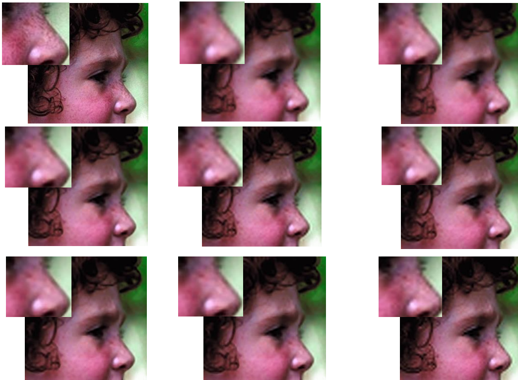
Fig. 7. Visual comparison: (Top-left) Original HR image, (top-middle) Bicubic, (top-right) SCSR[12], (middle-left) SISU[13], (middle-middle) GR[33], (middle-right) ANR[33], (down-left) AMSRR[24], (down-middle) SDS [25], (down-right) proposed POSR, magnification factor m=4 .
