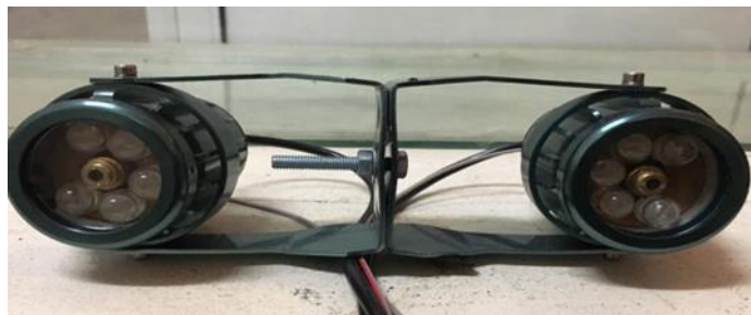
Figure 3. Light source structure and LEDs in different spectrums
