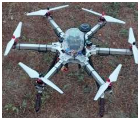
Fig. 4. A hexacopter drone developed for delivery plan.
